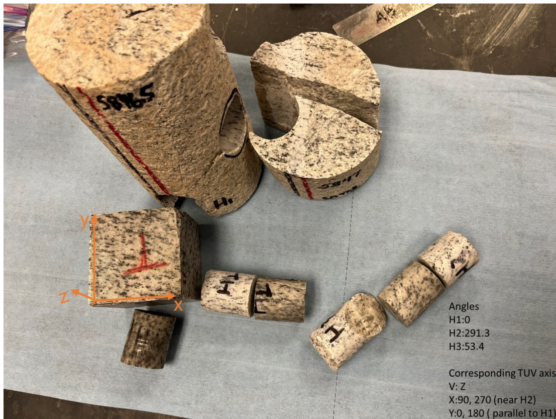
Figure 18: Lower Granitoid sample preparation for TUV sample (cube) with DRA samples (cylinders), showing x, y, z axes on TUV sample and with cylinders laying in approximate directional correspondence to TUV sample. The TUV sample was cut from the core section in the top of the image and the needle-like crystal elongation that is subparallel to the x-axis of the TUV sample is visible in both the TUV sample and the parent cores.
