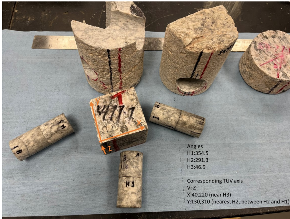
Figure 13: Upper Granitoid sample preparation for TUV sample (cube) with DRA samples (cylinders), showing x, y, z axes on TUV sample and with cylinders laying in approximate directional correspondence to TUV sample. The TUV sample was cut from the core section in the upper right, and the slight elongation of crystals in y-direction can be seen from the top of the core.
