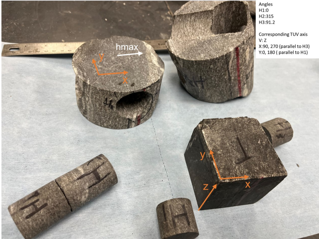
Figure 21: Upper Gneiss sample preparation for TUV sample (cube) with DRA samples (cylinders), showing x, y, z axes on TUV sample and with cylinders laying in approximate directional correspondence to TUV sample. The TUV sample was cut from the top of the image and the foliation that is subparallel to the core axis is visible in this parent core. The proposed orientation of the maximum horizontal stress is indicated on the surface of the top-left parent core.
