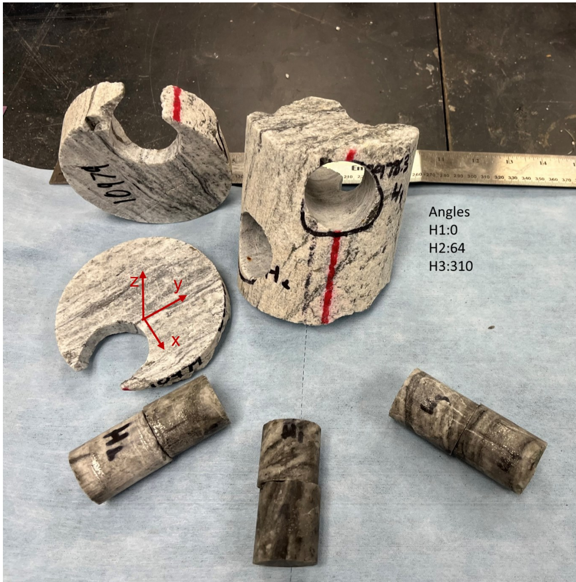
Figure 25: Parent core for Lower Gneiss with DRA samples (cylinders), showing x, y, z axes and with cylinders laying in approximate directional correspondence to TUV sample.
